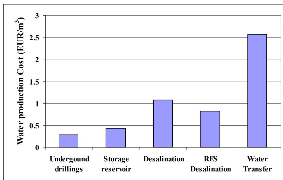
**Figure 2. Comparison of the water production costs for alternative water supply options**
