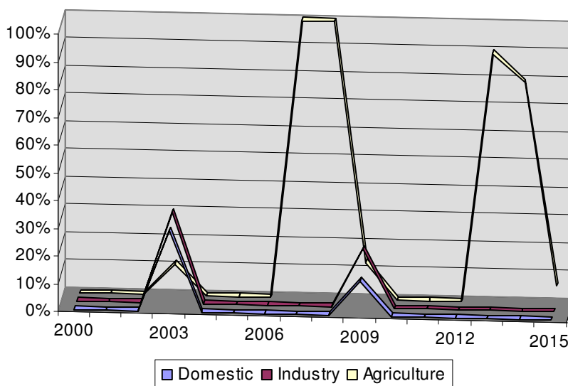
Figure 11-22 Percent improvements of deficit in domestic, industrial and agricultural uses under the BauC+R scenario relative to the reference BauC scenario
