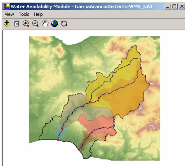
**Figure 4. The sub-basins generated by the pro-processor of the availability module using climatic data**
