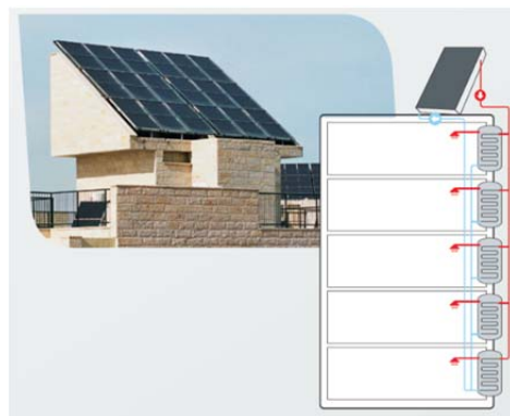
Figure 16 Central water heating installations with large storage tanks (Chromagen)
